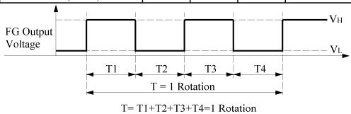
$$T=\frac{T1+T2+T3+T4=1 \text{ Rotation}}{T=\frac{60}{\text{rpm}}}$$
